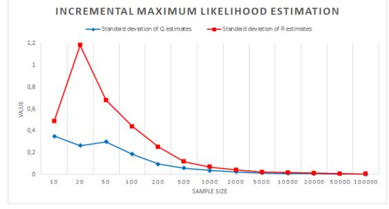
Figure 4: The same runs of Algorithm 1 as in Figure 3. Standard deviations are plotted against a sample size of 10, 20, 50,  $10^2$ ,  $2 \cdot 10^2$ ,  $5 \cdot 10^2$ ,  $10^3$ ,  $2 \cdot 10^3$ ,  $5 \cdot 10^3$ ,  $10^4$ ,  $2 \cdot 10^4$ ,  $5 \cdot 10^4$ ,  $10^5$ .
