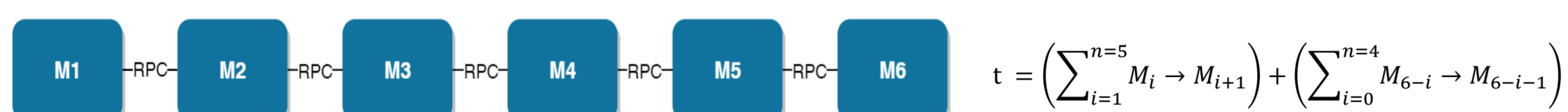
Fig. 1. The topology of microservices and formula used for the experiment.
