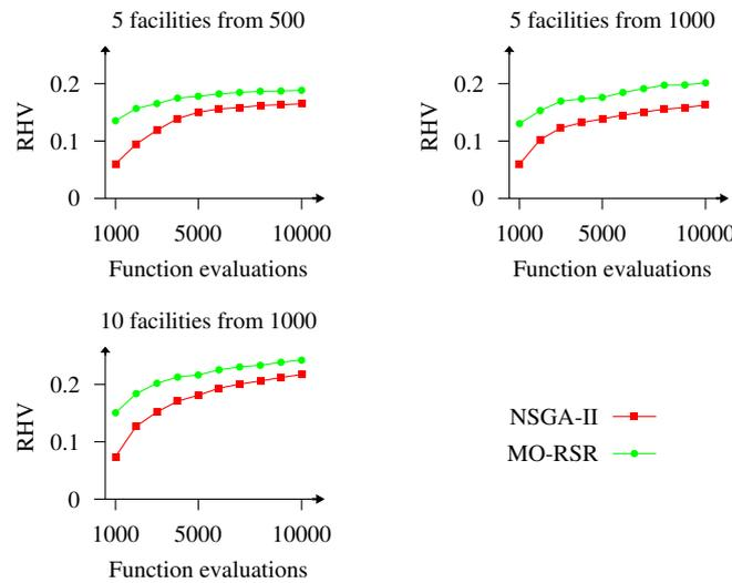
Fig. 4. Average results obtained by MO-RSR and NSGA-II for CFL/FE when selecting locations for 5 and 10 facilities from the set 500 and 1000 candidate locations.
