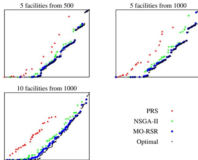
Fig. 5. Selected approximations of the true Pareto fronts, obtained by different algorithms, in the context of the true Pareto front.
