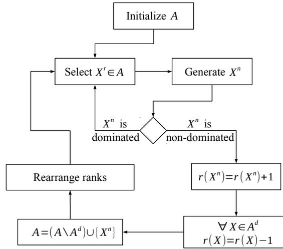
Fig. 1. Scheme of MO-RSR algorithm.
